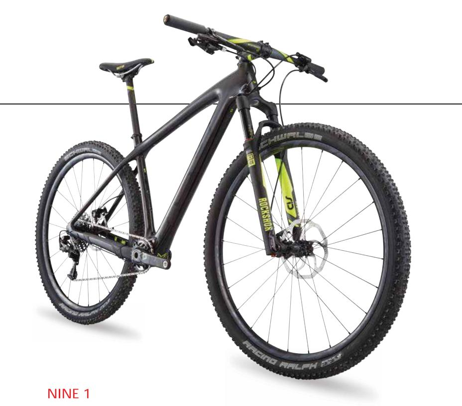
FRAME: UHC Advanced + TeXtreme® carbon FORK: RockShox Sid RL, 100mm COMPONENTS: SRAM X01
