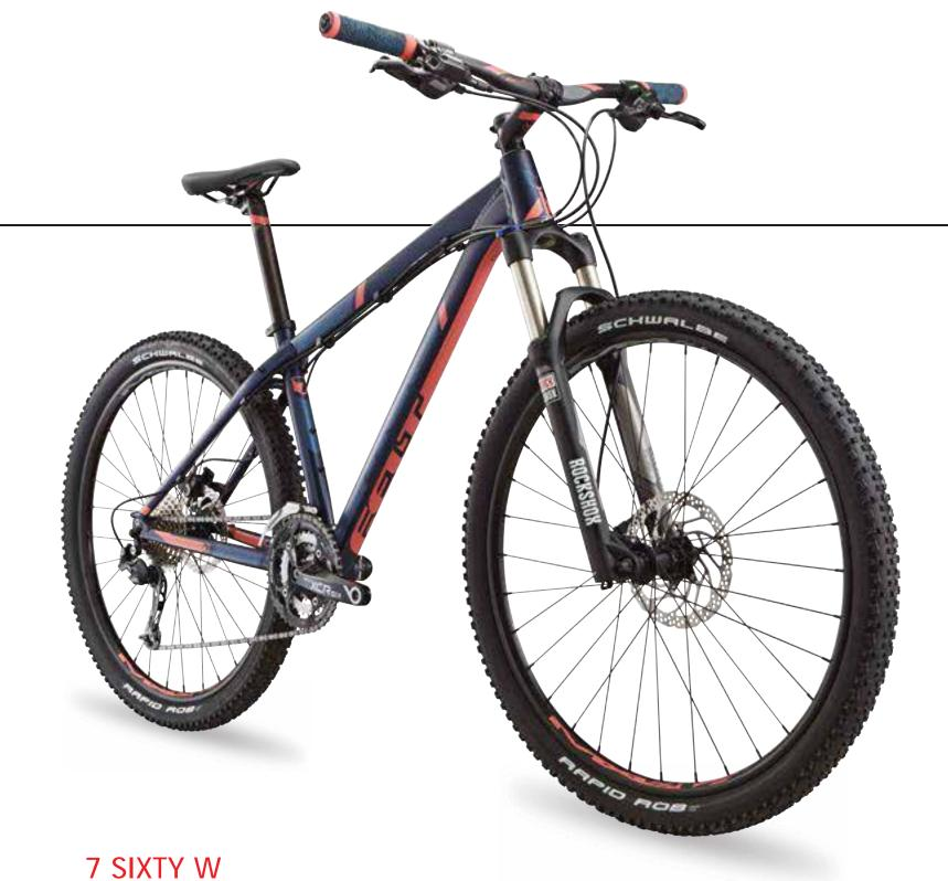
FRAME: Hydroform butted 6061 aluminum FORK: RockShox XC30, 100mm (80mm/XS) COMPONENTS: Shimano Deore/Acera
