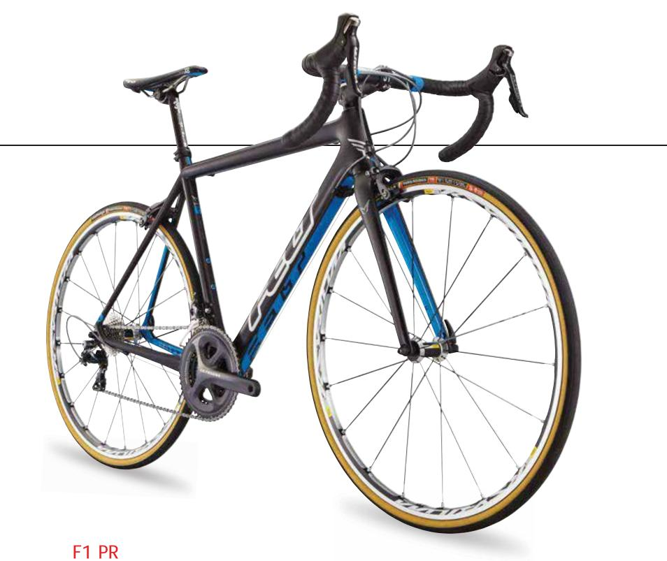
FRAME: UHC Ultimate + Nano carbon FORK: UHC Ultimate carbon COMPONENTS: Shimano Dura-Ace/Ultegra
