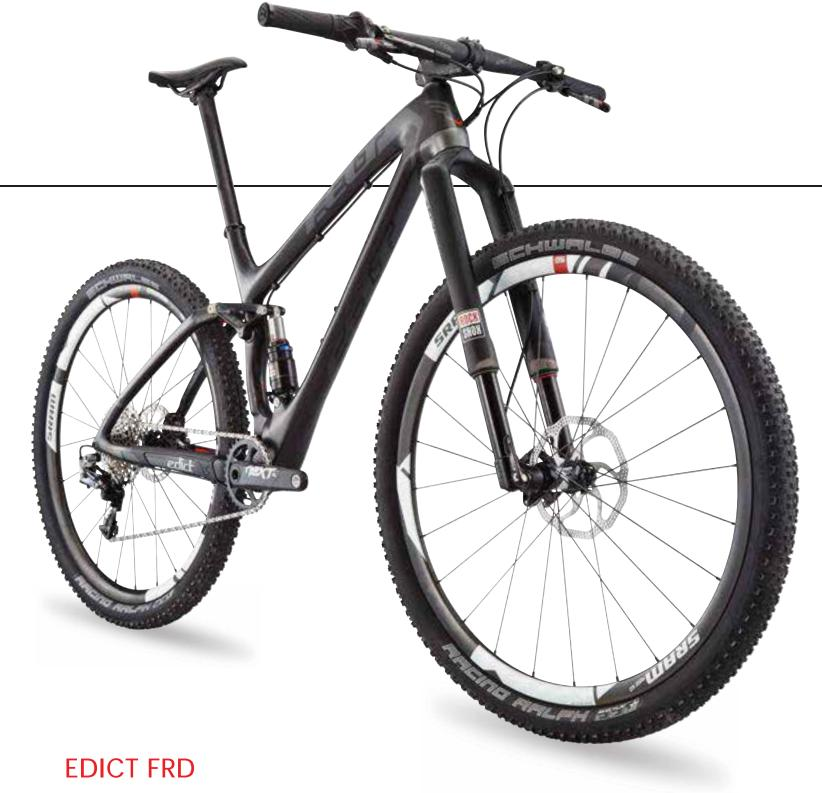
FRAME: UHC Ultimate + TeXtreme® carbon w/ FAST® FORK: RockShox RS1, 120mm COMPONENTS: SRAM XX1 Grip Shift
