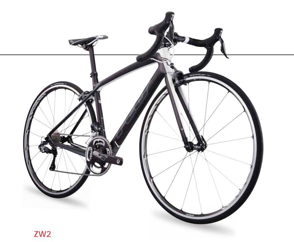
FRAME: UHC Performance carbon FORK: UHC Advanced carbon COMPONENTS: Shimano Ultegra Di2
