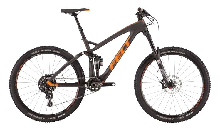
FINISH Matte Textreme (Orange) FRAME Felt Trail, UHC Advanced + TeXtreme carbon fiber, MMC w/ InsideOut construction, Full carbon dropouts, 140mm travel, FAST suspension, ControlTaper head tube, post disc mount, replaceable derailleur hanger, standard 73mm threaded bottom bracket, 12 x 142mm w/ Syntace style thru axle, internal derailleur cable/brake hose/dropper
