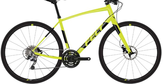
FRAME Felt Verza Speed, Superlite Butted aluminum, smooth TIG welding, flat mount disc standard, replaceable derailleur hanger
