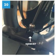
Gently snug fender to the lower bridge of the frame by locating the hole found on the back side of the motor assembly. You will need to use the supplied spacer to keep the fender the correct distance from the frame and tire.
