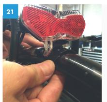
Adjust the fender to rough final position and use your fingers to bend the clamps found below the rear light so that they grip the fender.
