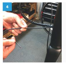
Once the front light cable has been separated from the main cable cluster, re-coil the cover back over the main cables.
