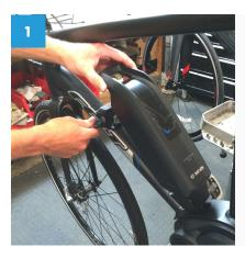
Start by removing the battery from the bicycle to ensure that the Bosch System is deactivated.
