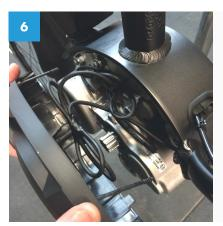
Remove the left side of the motor cover to expose the remainder of the rear light cable. Unbundle the rear light cable.
