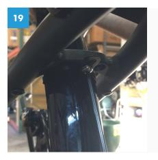
Hold the rear fender loosely in place and gently snug the fastening bolt into the bridge found under the seat stays.
