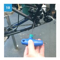
Begin installing the rear rack by snugging the lower mounts of the rack to the mounts found on the rear triangle of the bike.
