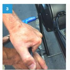
Begin removing the left crank arm by unthreading the left lock bolt.
