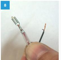
Keep the silicone cover in place while installing the cable crimp.
