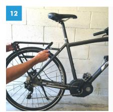
Place the bike on a flat surface and adjust the rear rack to make sure it is parallel with the ground.
