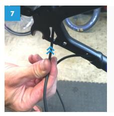
Grasp the rear light cable and pull the newly unbound cable to the rear end of the bike.
