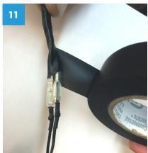
Once each of the wires are connected, tightly wrap the connections in electrical tape to protect them.
