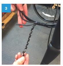
Carefully uncoil the front cluster of cables to expose the front light cable.
