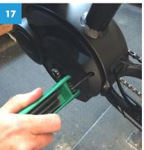
Reinstall the left side of the motor cover by carefully tucking the wires back in and tightening each of the 3 fastening screws.
