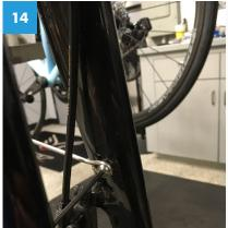
Insert the fender brackets into the mounts on the front fenders.
