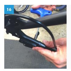
Reinstall the kickstand and then place both the front and rear wheel back on the bike.
