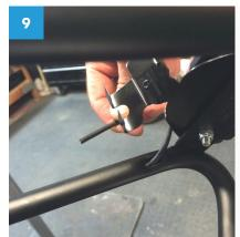
Once the cable has been threaded through the rack, carefully pull enough cable through to reach the rear light located at the top of the rack.
