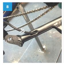
Thread the rear light cable through the opening found near the lower mount of the rack (non-drive side).
