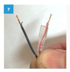
Once each of the cables are stripped, place a silicone cover over one of the wires.
