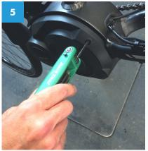
Remove each of the 3 torx screws holding the left side of the motor cover in place.
