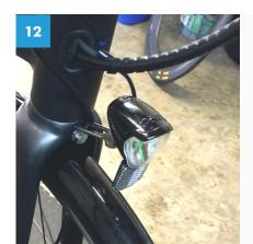
Tuck the excess cable back into the frame.
