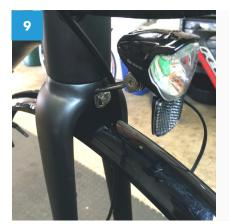
Loosely install the fender & front light by bolting them into the fork crown. Once in place, gently snug the fastening bolts.
