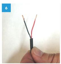
Strip each of the wires to allow for enough room for the cable crimps and silicone covers.
