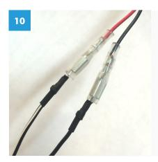
Connect the light wires to the Bosch System and slide the silicone covers over the connections.
