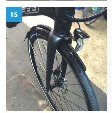
Once both brackets are loosely in place, reinstall the front wheel & adjust the front fender until the wheel no longer rubs. Once this is done, secure the fender by tightening each of the fender's fasteners and mounting bolts.
