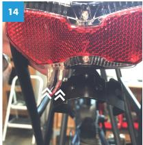
Once the wires have been prepped, plug each of the wires into the rear light and push the silicone covers up and into place.
