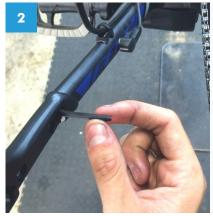
By removing the kickstand, you will be exposing the cable for the rear light.
