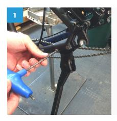
Move to the back of the bike and remove the kickstand, and set it aside.
