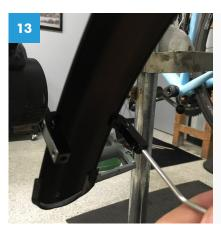
Gently snug the front fender bracket to the hole found on the inside of the fork blade. Do not tighten yet because you want to leave room for later adjustment.
