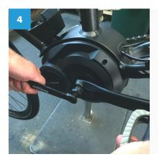
Once the left lock bolt is removed, use a crank arm puller to remove the left crank arm.
