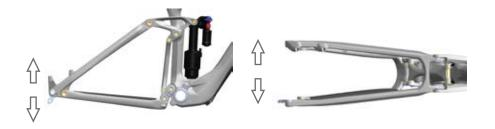
3. With the shock removed, move the suspension through its travel. There should be little to no resistance. If there is any resistance, please refer to the technical section for more information and instructions for bearing removal/installation.
