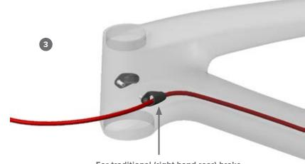
For traditional (right hand rear) brake lever setups, use the 2-hole 5mm port (ccn099yb) on the left side
