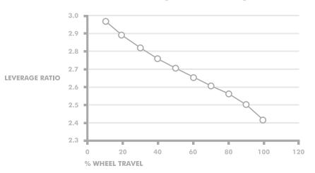
**Small-Bump Sensitivity** // For small-bump sensitivity, the shock is tuned with very little compression damping. Because the linkage is providing the pedaling efficiency and large impact support, the shock can remain active and absorb bumps when needed. The added benefit of doing this is the shock is not compensating for any shortcomings of the linkage design, therefore it is not working as hard which leads to less heat buildup and more consistent performance.
