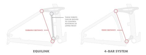
**Efficient Pedaling //** To accomplish efficient pedaling, the suspension is designed with an ideal amount of anti-squat. A key benefit of the Equilink is that it allows for a downward sloping anti-squat curve which falls off more rapidly around 60% travel. This translates to a bike that pedals well and is able to absorb bumps at the same time.
