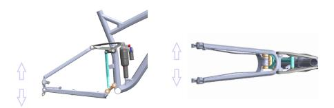
3. With the shock removed, move the suspension through its travel. There should be little to no resistance. If there is any resistance, please refer to the technical section for more information and instructions for bearing removal/installation.
