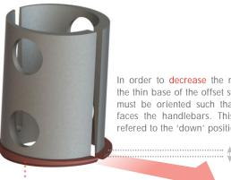
In order to decrease the rise, the thin base of the offset shim must be oriented such that it faces the handlebars. This is refered to the 'down' position.
