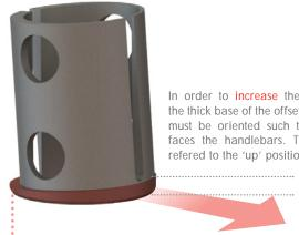
In order to increase the rise, the thick base of the offset shim must be oriented such that it faces the handlebars. This is refered to the 'up' position.
