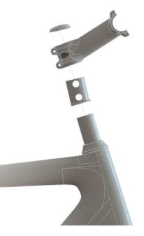
First. Insert the appropriate shim in the up or down position
