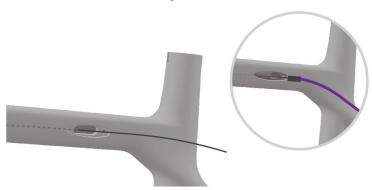
Feed cable through the top tube until cable exits rear top tube grommet nearest to the seat tube. C: Replace the top tube grommet and tighten the 2mm screw to secure in place as shown.
