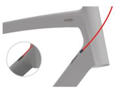
A: Feed Front Derailleur Cable into Mousetail C: Repeat the pre-Ferrule and downtube via Cable Stop as pictured. Derailleur Cable. Pull cable taut as it exits the bottom bracket hole.
