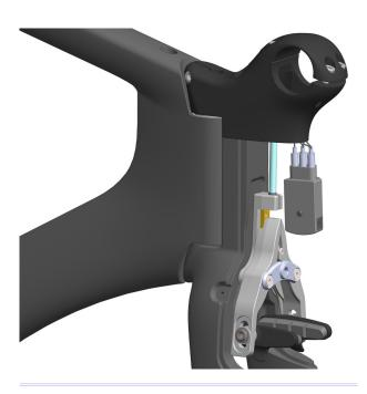
Once the Di2 wires are plugged into the junction box, begin to organize the wires and box to create a package that will fit underneath the cover.
