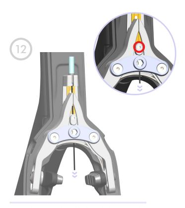
Thread the Front Brake Cable through the Front Brake Cable Housing, through the Barrel Adjuster and into the Front Brake as shown.
