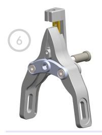
Install Carriage Assembly followed by installing the Front Plate and tighten screws to 2Nm.
