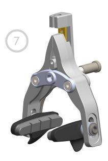
The brake pads can now be installed finishing the brake assembly. The brake is now ready to be re-installed on the fork.
