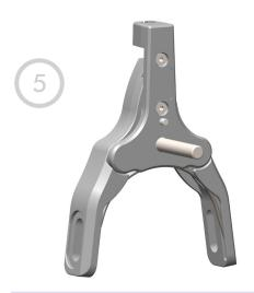
Add Bushings to Brake Arms. Slip Brake Arm and Spring Pre assembly onto Brake Posts. Add Brake Mount Bolt.
