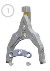
Remove Front Plate and Mounting Screws.
