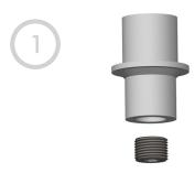
Start by assembling the steerer nut & the steerer lock screw. Be sure to use an anti-seize compound on the aluminum threads to prevent seizing and gaping.
