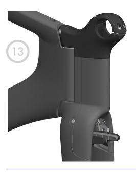
Place cover on and secure with M3 bolts. Tighten each bolt to 2Nm.
