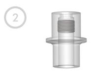
Using a 6mm allen key, thread the steerer lock screw into the shaft nut in until it hits the top of the shaft nut. Do not tighten the steerer lock screw down. You are simply moving it out of the way for later installation.
