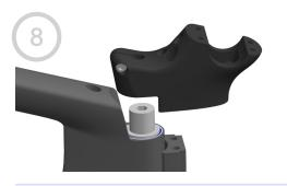
Install the Bayonet stem by placing it over the steerer shaft nut.
