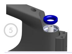
Apply grease or an anti-seize compound to the upper bearing race of the frame and slide the upper headset bearing down the steerer tube until it is firmly seated in the bearing race in the frame.
