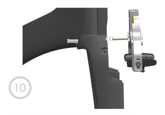
Fasten the Front Brake to the fork using the Brake Mounting Bolt and the 30mm Brake Mounting Nut and Serrated Nut as shown.
