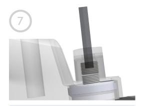
Insert a 6mm allen key through the opening found in the steerer nut and into the steerer lock screw. Turn the steerer lock screw clockwise until it contacts the steerer shaft. The steerer lock screw locks the headset adjustment. Tighten this to 5Nm with a torque wrench.
