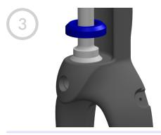
Apply grease or an anti-seize compound to bearing race located on the fork. Then proceed to slide the lower headset bearing into place on the steerer tube.
