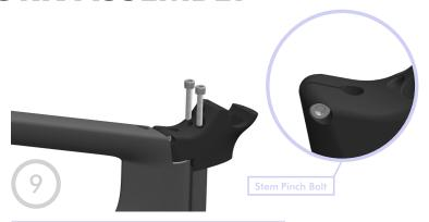
Insert the M6x40mm bolts through each hole in the stem. Thread each bolt into the holes in the bayonet fork. If the threads don't engage, shift the stem until correctly aligned. Tighten the two bolts to 12Nm then tighten the pinch bolt to 5 Nm.
