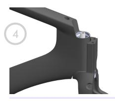
Guide the steerer tube through the head tube of the frame until the bearing seats into the bearing race in the frame.
