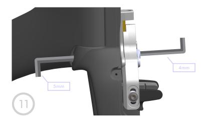
Using a 4mm and 5mm Hex Wrench, tighten the Brake Mounting Nut and Bolt to 6Nm.
