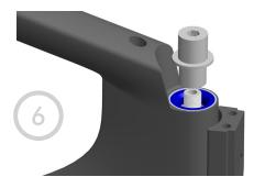
Apply grease or an anti-seize compound to the bearing race found on the steerer shaft nut and the threads on the steerer tube. Then proceed to thread the steerer shaft nut onto the steerer tube. Use 8mm Allen Key to tension the headset like you would on a standard threadless headset. Do not over tighten.
