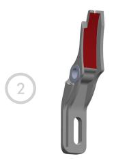
Apply a thin film of light waterproof grease to Brake Arm Cam surfaces.
