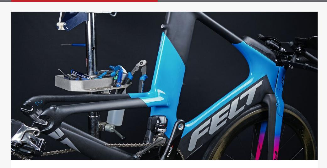
**Step 1:** Remove the rear wheel to simplify the installation.
