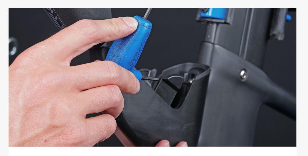
**Step 3:** Slide the box up over the top screw post. Insert the top screw and tighten to 4Nm.
