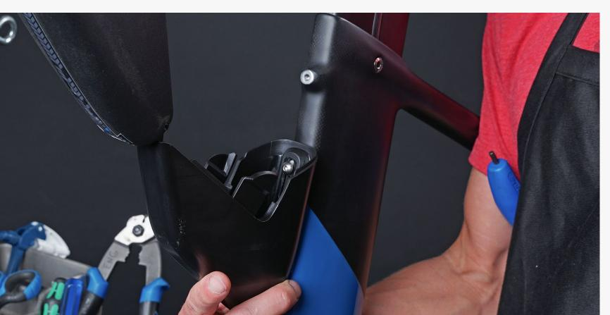
**Step 2:** Install the lower screw. Turn 3 or 4 revolutions.
