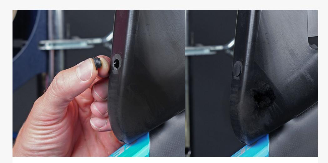
**Step 5:** Insert the supplied plug in the hole to seal it.
