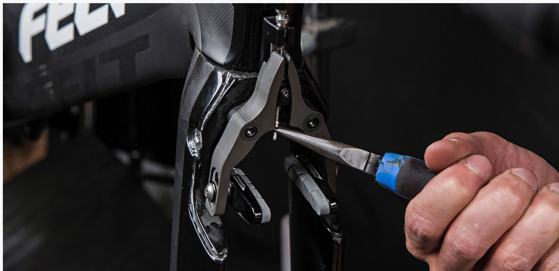
Step 17: Install cable end.
