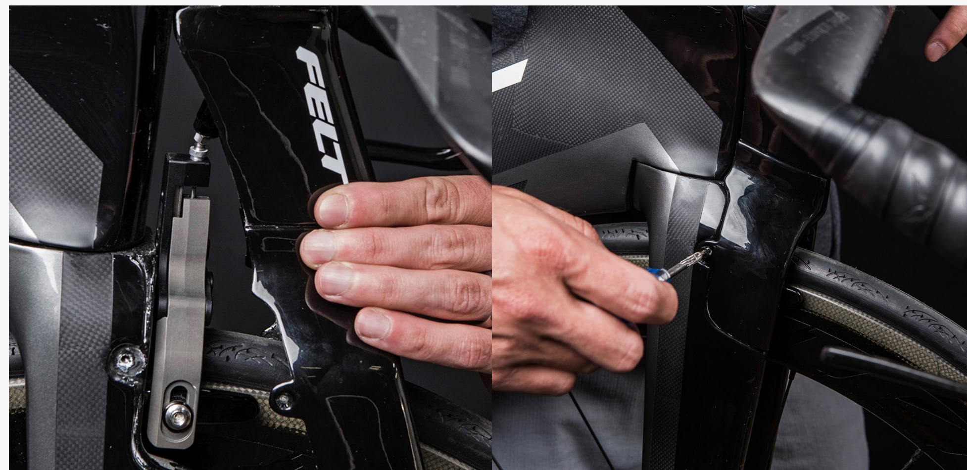
Step 20: Install the covers and tighten the (4) M3 screws to 4Nm. Finished.
