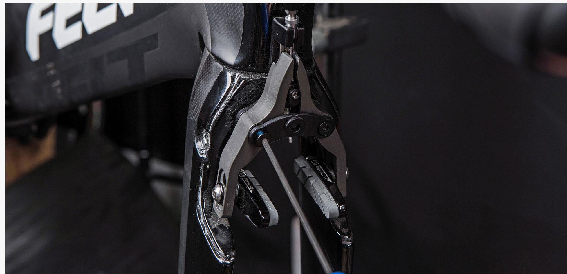
Step 18: Reinstall the front plate and tighten to 2Nm.
