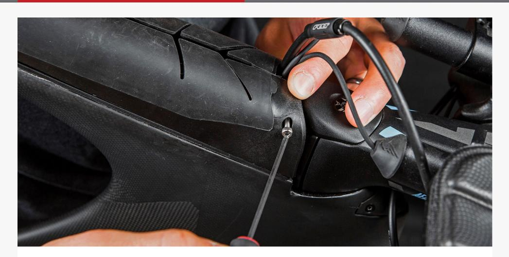
**Step 8:** Attach the front of the top of the CALpac together using the remaining 12mm M3 screw. As before, note that the screws are self-tapping, so great care must be taken on the first installation. Tighten to 2Nm.
