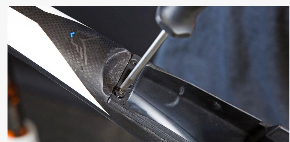
**Step 2:** Using a high-quality T9 Torx driver, remove the (7) screws that are attaching the box to the frame. Note that older IA and IAx models utilized Hex screws. Use a high-quality 2mm hex driver to remove those screws. DO NOT use a ball-end style driver. Do NOT throw away these screws as they are used in the latter installation step as well as in other applications on your bicycle.
