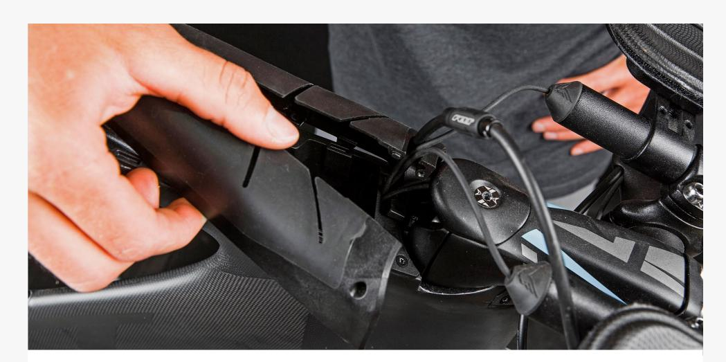
**Step 7:** While flexing the front of the CALpac apart, install it over the cables. Make sure that you correctly route the cables. Please refer to the diagrams below.
