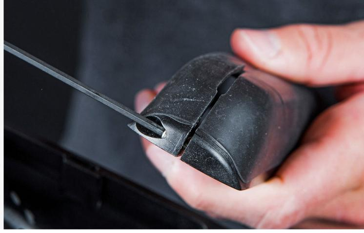
**Step 6:** Starting with the back screw, attach the two halves of the top of your new CALpac together using the shorter (12mm) of the two sized screws that are provided. Note that the screws are self-tapping, so be especially careful when screwing them in for the first time. Tighten to 2Nm. DO NOT install the front screw at this point.
