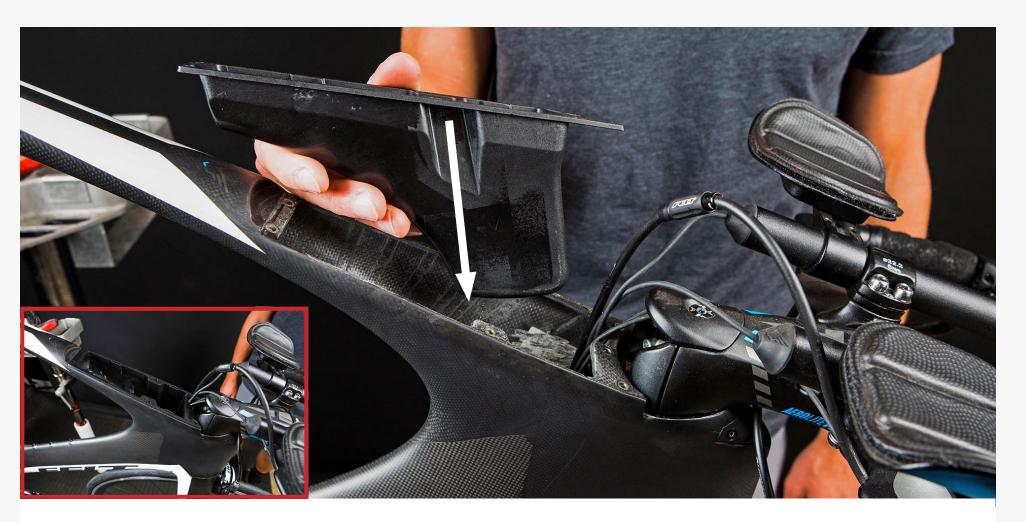
**Step 4:** Insert the new box in the direction shown above taking care to make sure that all of the cables entering the frame are routed in front of the CALpac and are not trapped on the side between the frame and the box.
