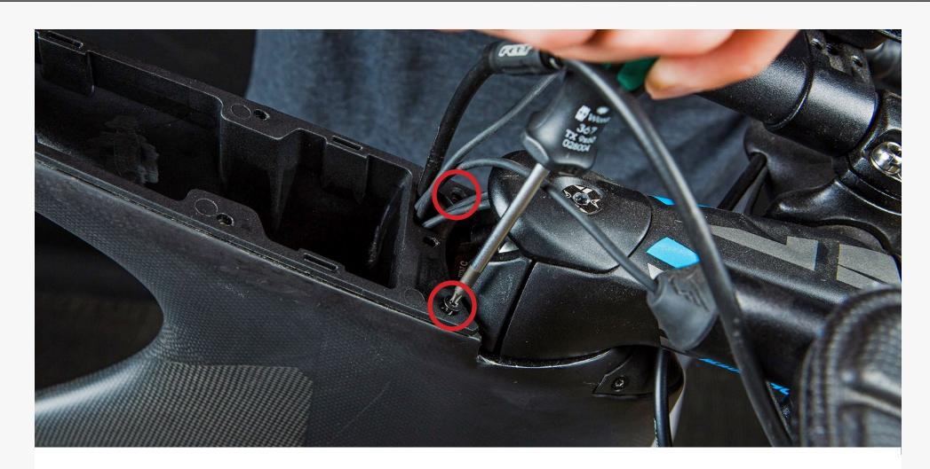
**Step 5:** Attach the CALpac to the frame with (2) M3 Flathead screws. Use the screws that you saved from step 2 or use the new screws provided with your CalPac. Install the two screws through the two front holes found on each side of the box. Use a T9 Torx driver or a Hex driver, if you have Hex screws, and tighten to 2Nm. DO NOT install the other screws yet.
