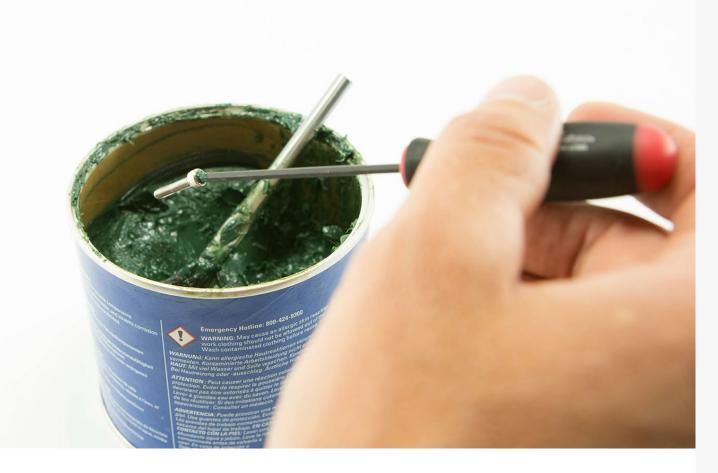
**Step 10:** To help install the remaining screw at the front of the CALpac, use a little bit of grease on the Hex driver to retain the screw as you insert it through the hole. Tighten to 2Nm.
