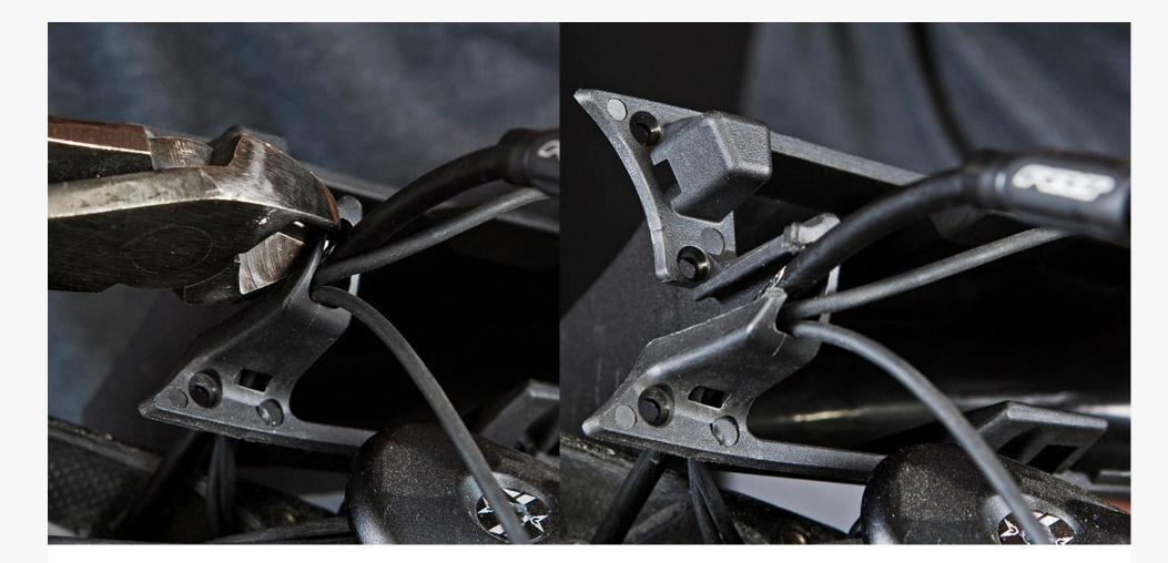
**Step 3:** If you prefer to leave the existing cable routing intact, use side cutters to cut out a slot in in the cable routing tower to free the cables.
