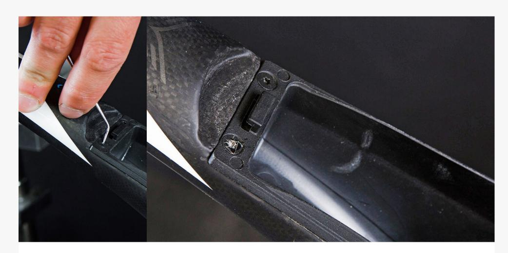
**Step 1:** One of the (7) screws holding the old CALpac has a protective adhesive covering the top of the screw. Carefully remove it using a sharp tool to expose the screw head.
