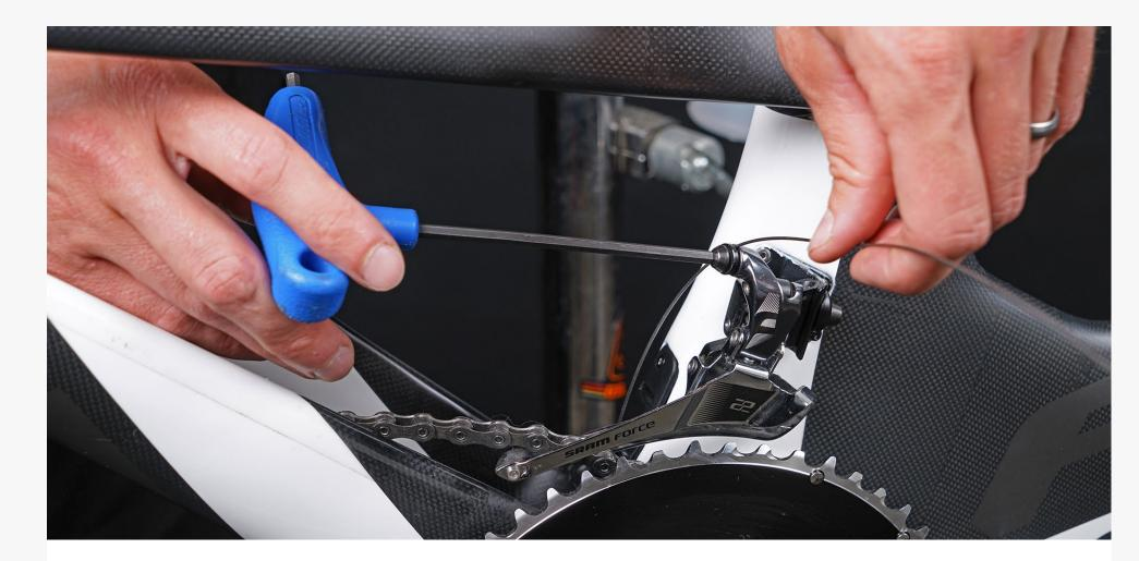
**Step 7:** Properly install the inner wire in the derailleur in accordance with your derailleur specifications.
