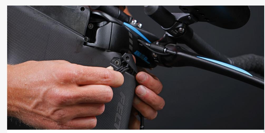
**Step 2:** If your Di2 wire length is limited, then you can first detach the Di2 wires from the A junction by using the Shimano Di2 installation tool while lifting the nose cone slightly out of the frame.
