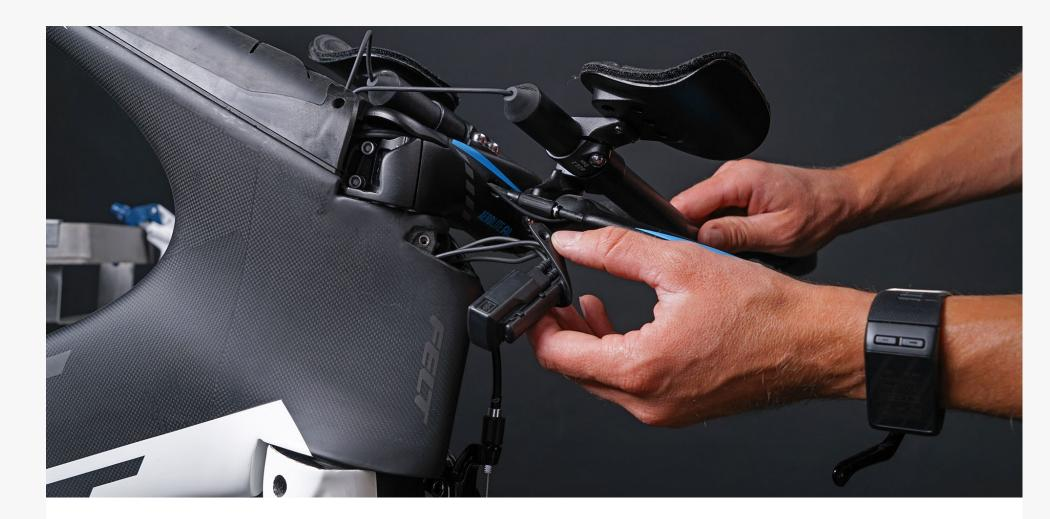
**Step 3:** Remove the nose cone.
