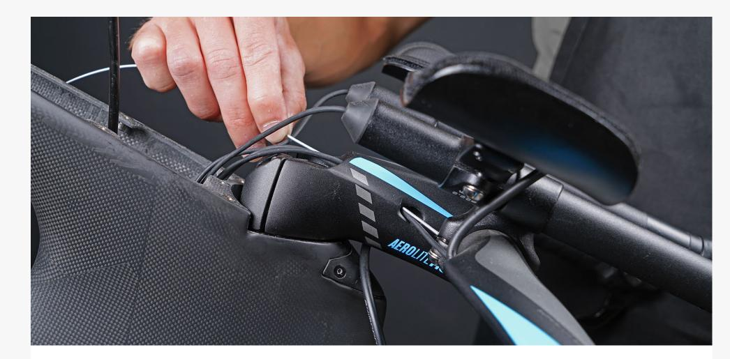
**Step 7:** To route the new housing through stem begin by inserting a spare inner wire from the back of the stem and through the side port entry hole.
