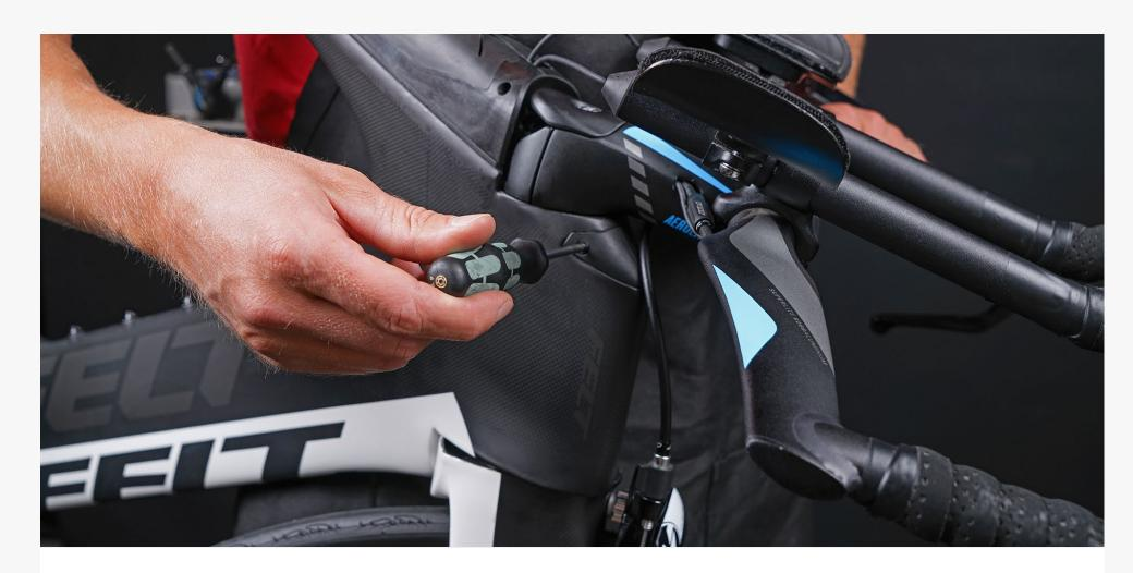
**Step 1:** Using a T9 Torx drive, unscrew the (2) M3 screws that attach the Di2 nose cone to the frame.
