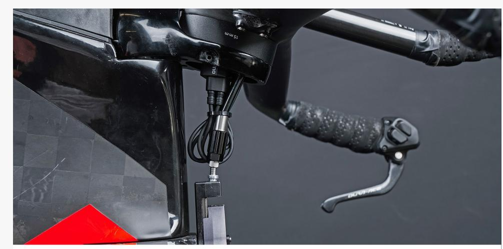
**Step 2:** The A junction is located under the upper brake cover.
