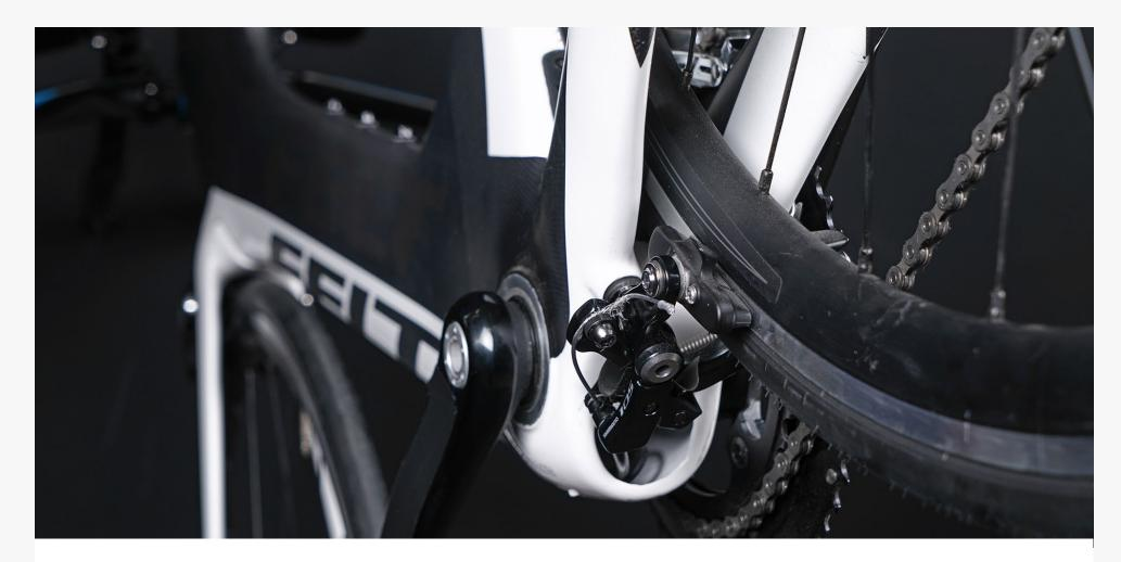
**Step 12:** Install the new inner wire in the caliper per your caliper manufacturer's instructions.
