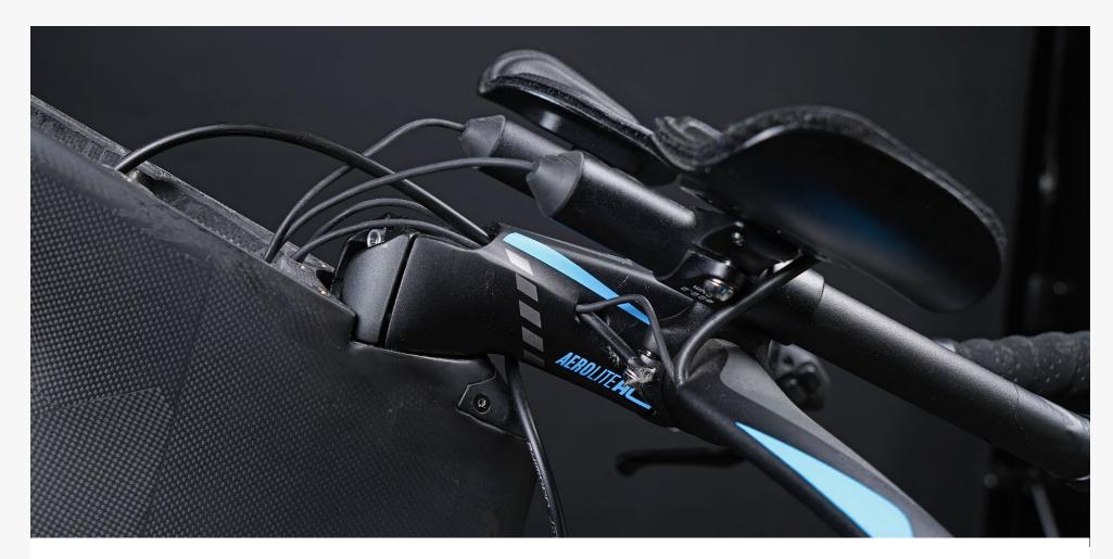
**Step 8:** Guide the housing that you inserted in Step 5 over the inner wire.
