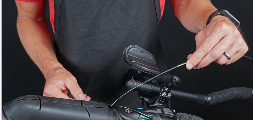
**Step B:** Pull out the cable housing while leaving the cable inside the frame. Use the cable in the frame as a guide to insert new housing.
