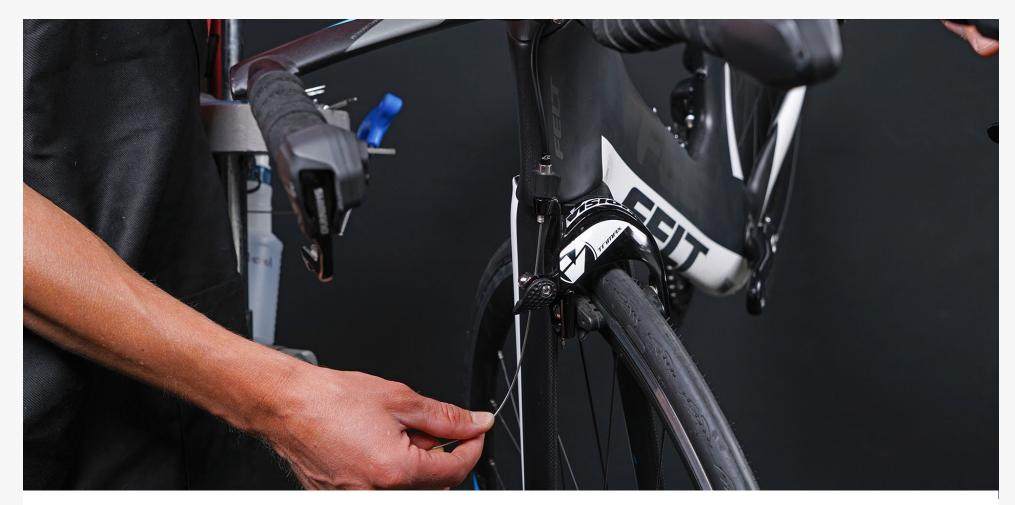
**Step 4:** Secure the inner wire in the brake caliper. Tighten to the specifications recommended by the caliper manufacturer. Trim the cable and install cable end.
