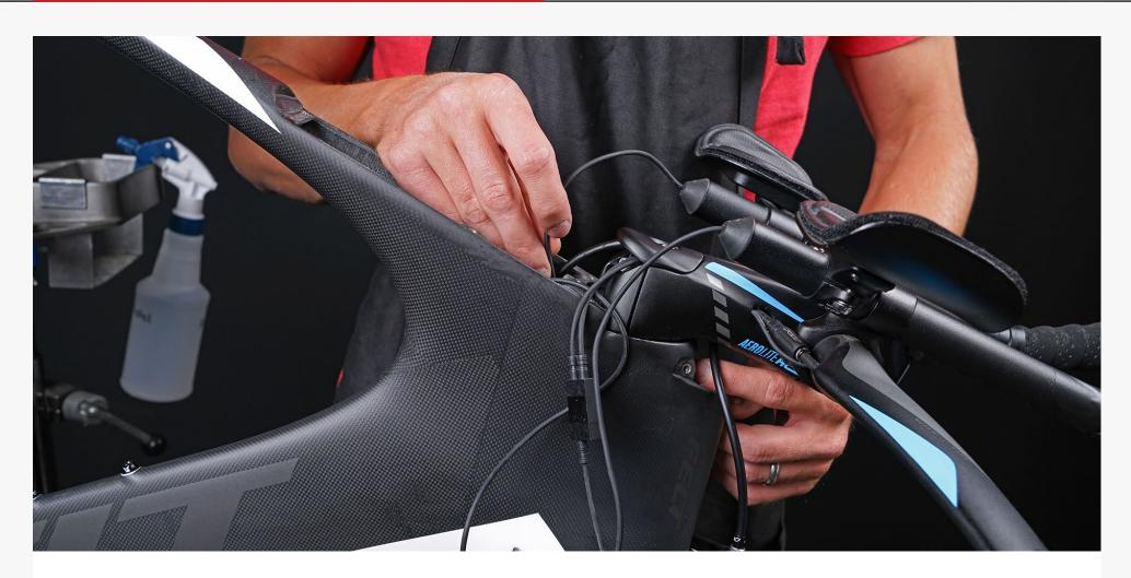
**Step 7:** To re-install Di2 wires, start at the frame opening and guide the cables around the steerer tube right below the top surface of the headtube. If you are not using Junction B to extend your shifter wires, then guide the shifter wires on the left side on the steerer tube. Otherwise, either side is acceptable. Do the same for brake wires and the single wire going down to the B junction by the bottom bracket.
