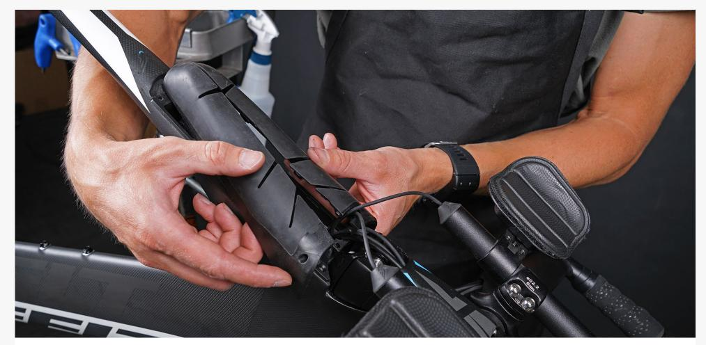
**Step 4:** Flex the two halves of the Calpac top outward to free from cables and remove.
