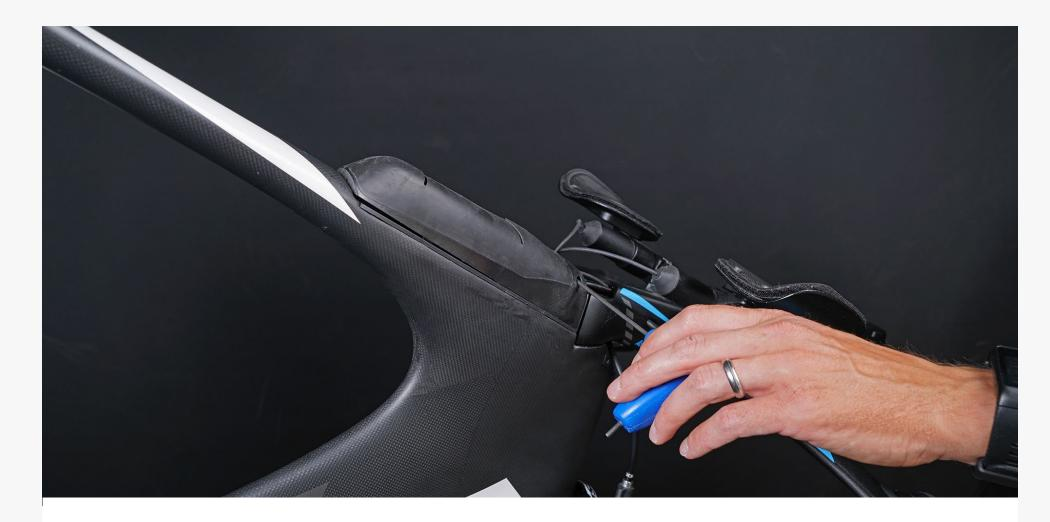
**Step 3:** Unscrew the front side screw on the side of the CALpac to separate the two halves of the box cover.
