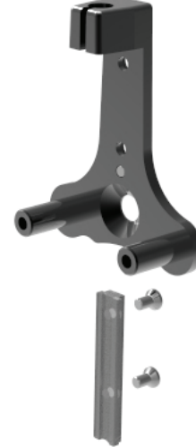
Step 6: Remove Track from Backing Plate.
